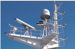
Marine radar antennas
