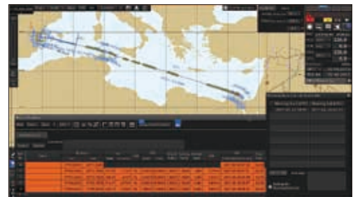
Example of Satellite Transmission Blocking Area Display
