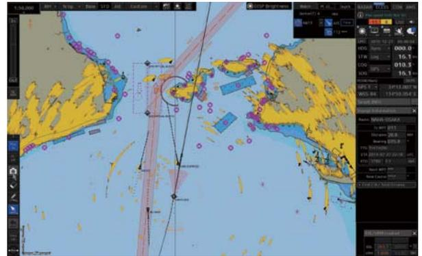
Example of additional display of radar overlay function
