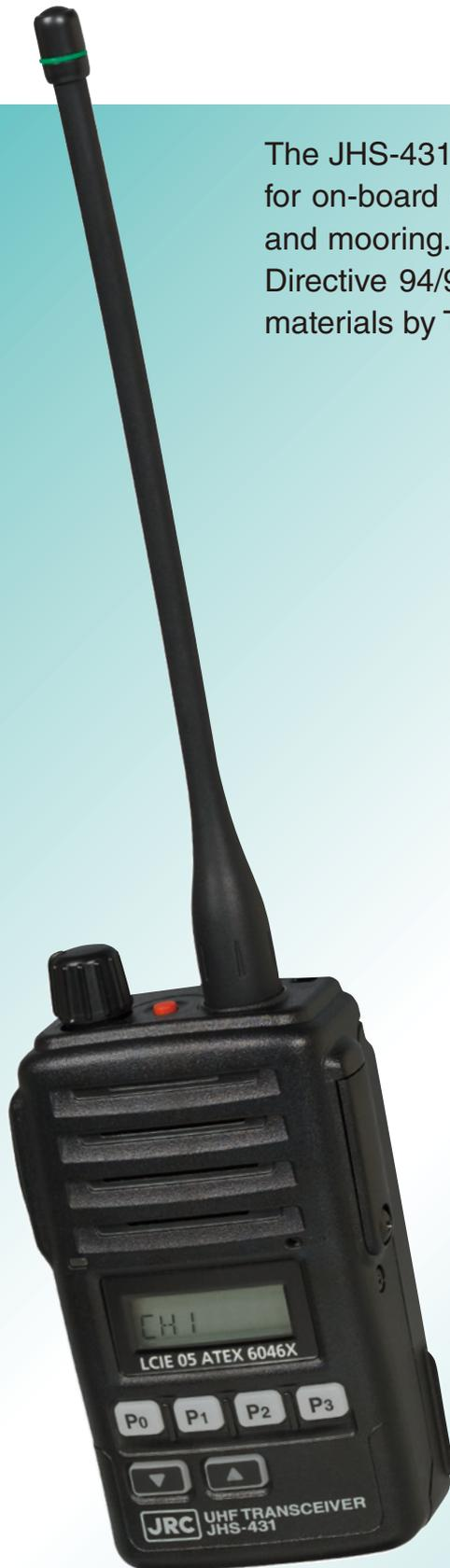
The JHS-431 is a 2 Watt UHF intrinsically safe transceiver designed for on-board communications in ship operations, loading/unloading, and mooring. The JHS-431's intrinsically safe structure meets ATEX Directive 94/9/EC for use when transporting flammable, dangerous materials by Tanker, LPG carrier, LNG carrier and/or LO carrier.
