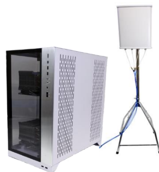
Figure 3: gNB (5G base station).
