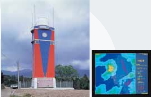
A small radar system capable of detailed measurements, even for local rain showers
