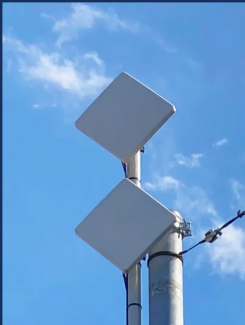
Directional antennas installed on the test course
